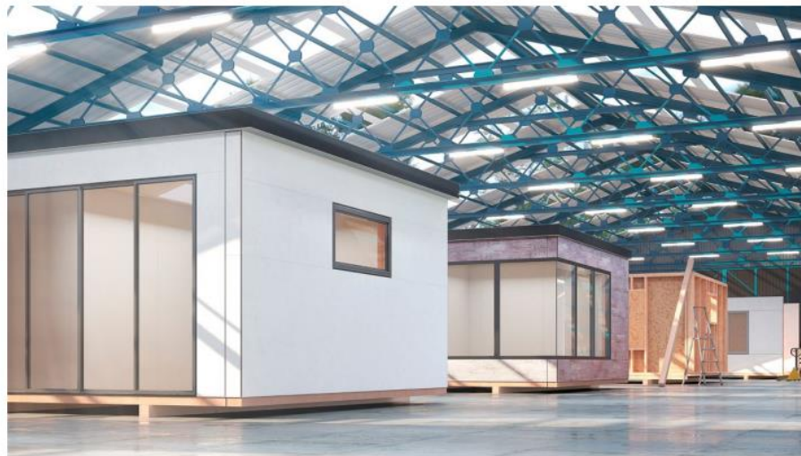
MMC homes in production and a completed scheme
