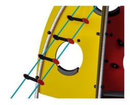
Ropes are made of UV-stabilised PA with inner steel cable reinforcement. The rope is induction treated in order to create a strong connection between steel and rope which leads to good wear resistance.
